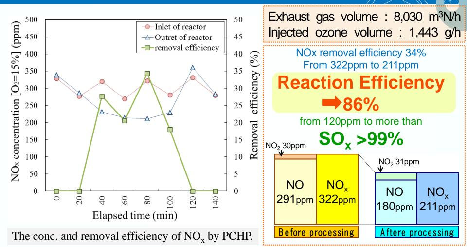
In wet type exhaust gas treatment system, it was concluded that application of the PCHP to an actual exhaust gas of glass furnace is highly effective.
