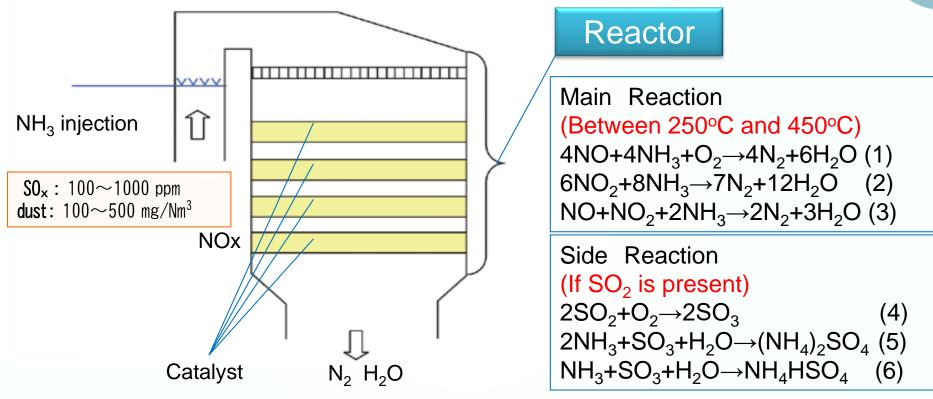
SCRThese side reaction, including dust develops<br/>catalyst poison and clogging problems.<br/> $\rightarrow$  SCR is difficult to use for de-NOx in glass<br/>melting furnaces.
