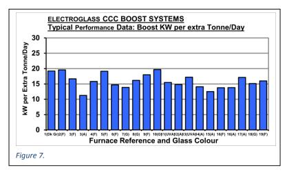
A well-designed electric boost system can melt 1 additional tonne per day of glass with a continuous power input of just 20 kilowatts and often less. Figure 7. shows the operating boost energy consumptions in a selection of 20 or so furnaces large and small. Each of these shows an actual boost energy consumption of 20kW or less per additional tonne per day.
