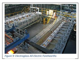
Figure 9. shows the two forehearths after their conversion to all-electric heating. On recommissioning, the electrical energy consumption of the re-designed forehearths quickly stabilised at 1535 kilowatt-hours per day for both, at a cost of 0.051 US\$ per kilowatt-hour or 5.1 US Cents per kilowatt-hour, and a daily electricity cost of US\$ 78.3, an extremely impressive 84% energy cost saving.
