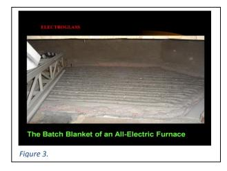
The very best of fuel-fired furnaces and heat recovery systems cannot compete with coldtop electric melting in terms of energy efficiency. Energy efficiency in this context means the proportion of the total energy used that actually goes into converting cold batch into fully molten and refined glass, the rest being lost to the environment in structural heat losses and combustion gases.
