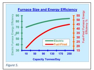
In contrast, a well-designed all-electric furnace of similar 250 tonnes/day capacity, which is at the top end of electric furnace experience, has a thermal efficiency of close to 85%, with just 15% of the total energy input being lost. These figures vary somewhat with cullet percentage in the batch mix, as re-melting cullet uses approximately 30% less energy than melting pure batch.
