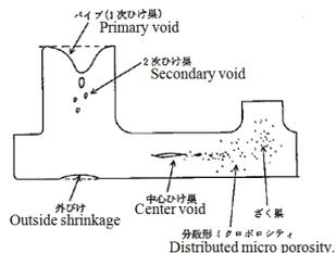
Fig.2 Internal defect in the field of casting metal. <sup>1)</sup>
