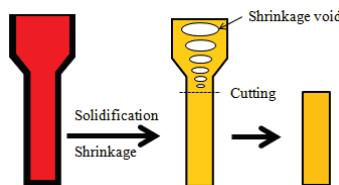
Fig.1 Manufacturing process of AZS refractory block
