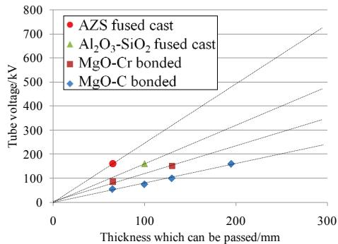
Fig.4 The relation between voltage and thickness which can be passed.
