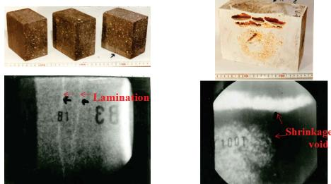
Fig.3 Internal defect inspection of some refractories by x-ray.
