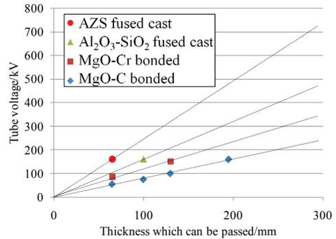
Fig.4 The relation between voltage and thickness which can be passed.
