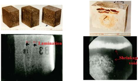
Fig.3 Internal defect inspection of some refractories by x-ray.
