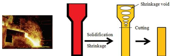
Fig.1 Manufacturing process of AZS refractory block
